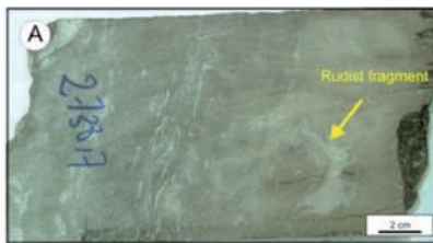
A- Bioclastic limestone with large rudist fragment within the top of BU1 (well B, core 11)
