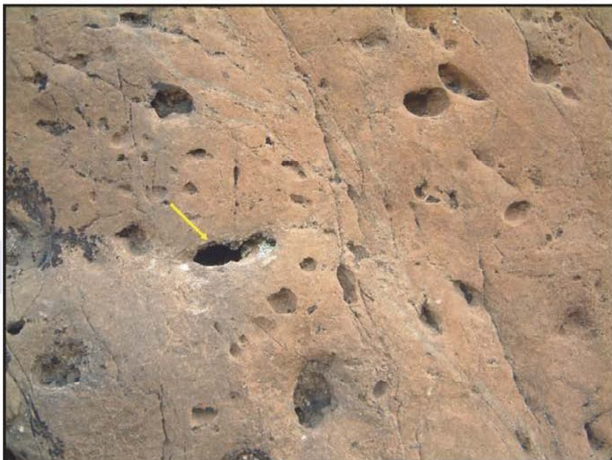
Photo B : Visible vuggy porosity within the third massive carbonatic unit (H3) of the Hameima Formation. The Jebel Bou El Hanèche section
